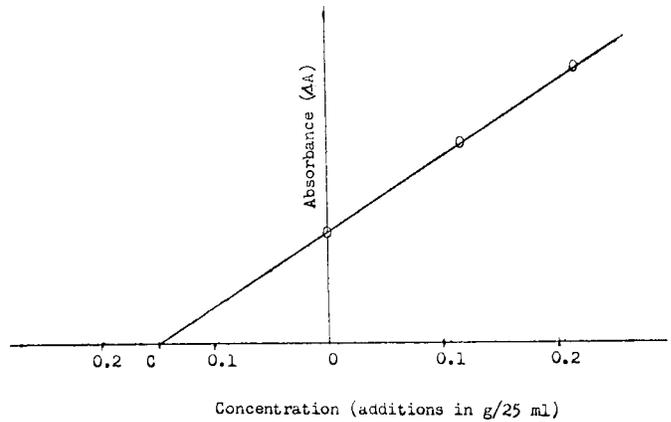
**FIG. 1 Plot of ΔA versus Cellulose Nitrate Additions**
